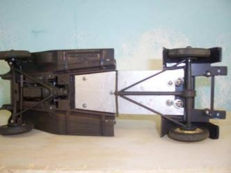
This vehicle started life as a Pick Up truck, it was cut behind Cab, lengthened & re-joined.
